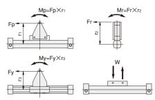
Pitching moment : Mp=Fp $\times$ r<sub>1</sub>....... 1N·m [0.74ft·lbf] Rolling moment : Mr=Fr $\times$ r<sub>2</sub>...... 0.2N·m [0.15ft·lbf] Yawing moment : My=Fy $\times$ r<sub>3</sub>..... 0.3N·m [0.22ft·lbf] Maximum load capacity : W...... 20N [4.5lbf.]
